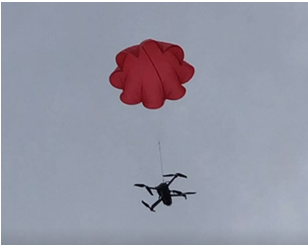
Figure 7. Parazero Safety System Test
