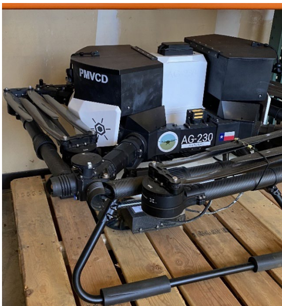
FIGURE 5A. PHOTO OF TWO HOPPERS MOUNTED IN THE AG-230 DRONE
